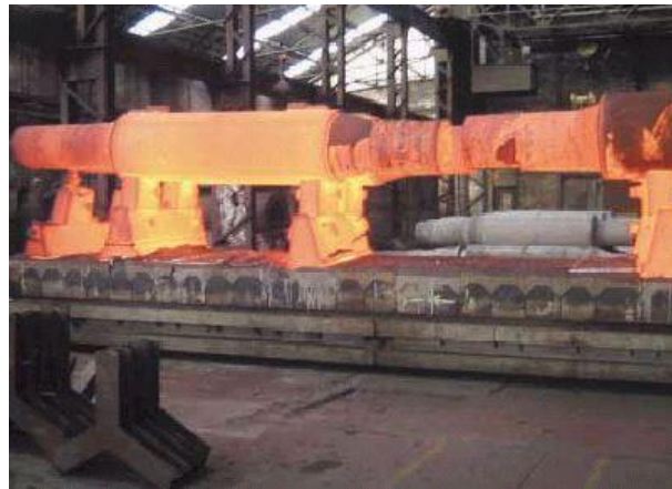
Figure 1 : A roll after heat treatment in Marichal Ketin Industry. [25]
